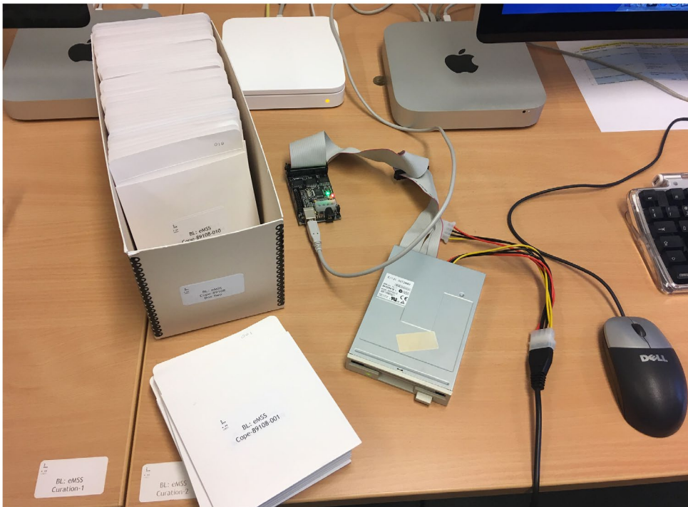
Figure 1. Capturing 3.5-inch floppy disks using Kryoflux.
